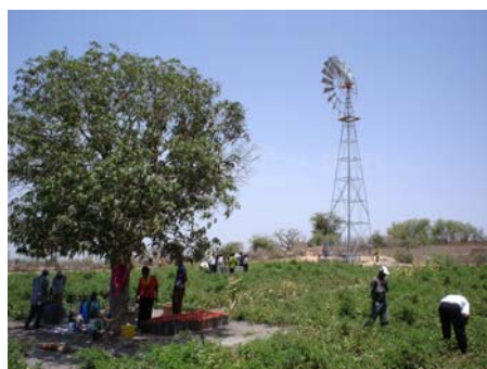
Irrigation by a windmill driven pump, Senegal
